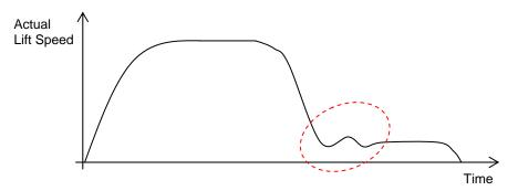
This effect can be eliminated by selecting the "Custom" setting for the deceleration (5-7 for up, 6-7 for down). The Custom value is then adjusted in the advanced parameters (menu 9 on the hand held programmer).
